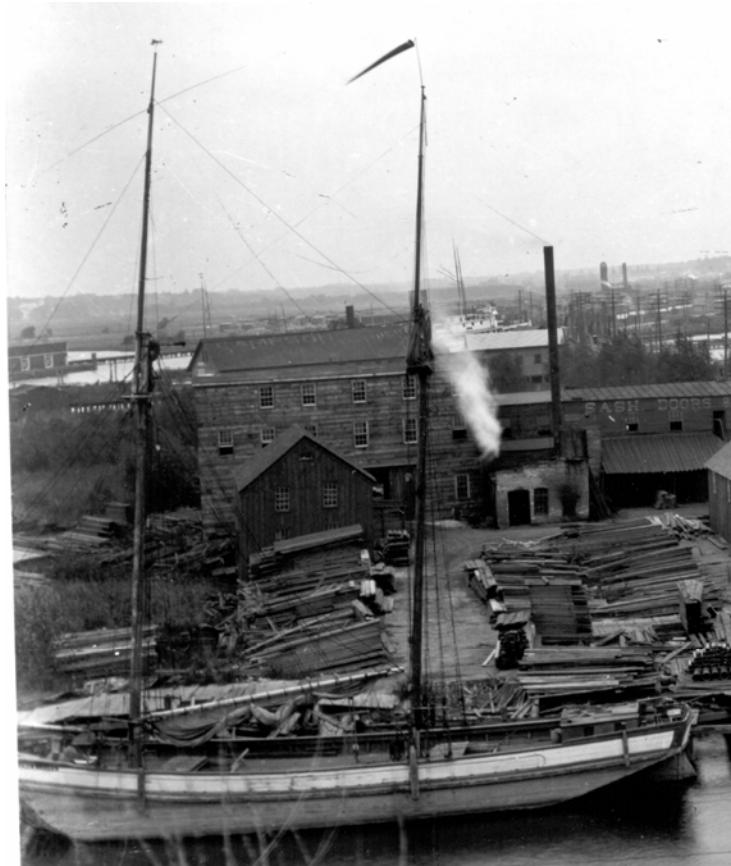
Figure 42. *Tennie and Laura*, date and location unknown. Note scuppers along lower edge of white paint, as well as large rubbing strake just below white paint. Courtesy Historical Collections of the Great Lakes, Bowling Green State University.
